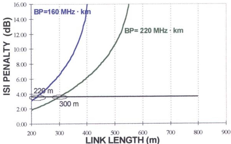
Figure 4. Measurements of overfilled bandwidth versus restricted mode launch bandwidth
