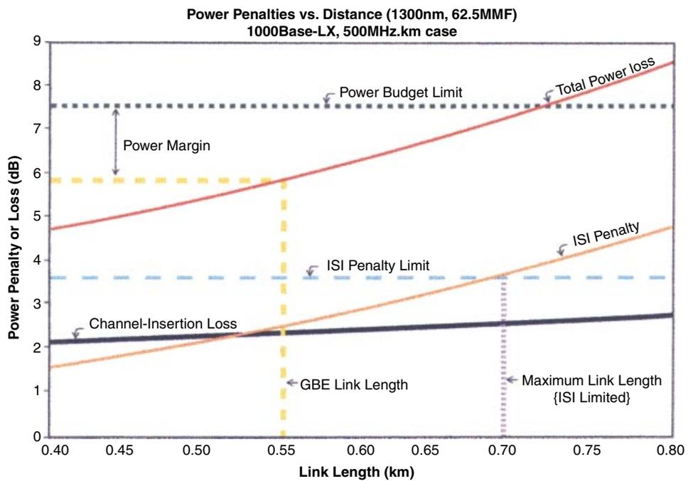
Figure 3. Power penalties versus distance (1300 nm, 62.5 multimode fiber)
