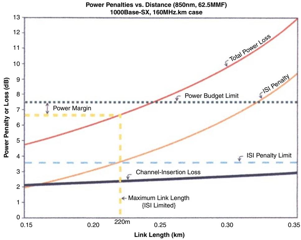
Figure 2. Power penalties versus distance (850 nm, 62.5 multimode fiber)
