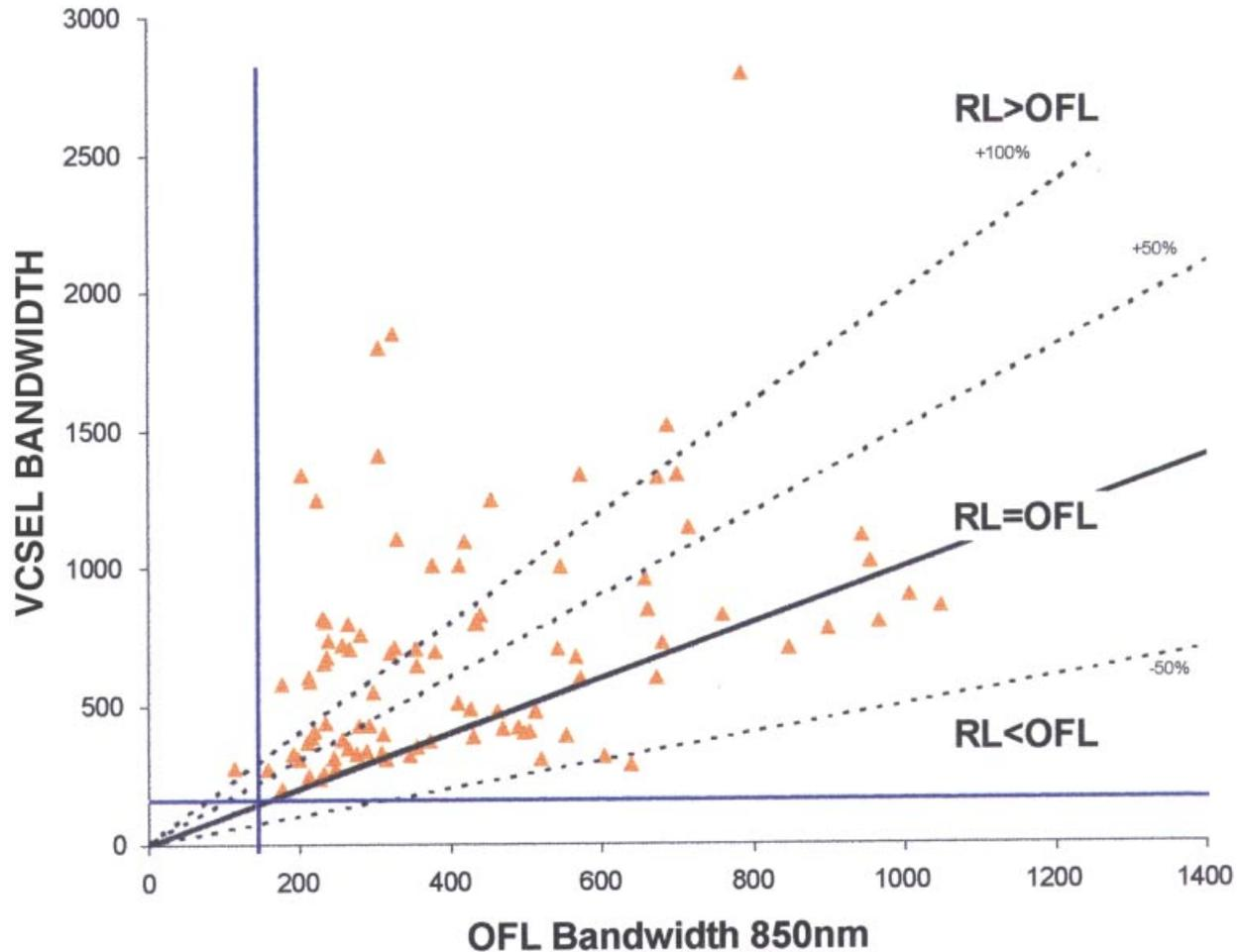
Figure 5. VCSEL bandwidth versus overfilled launch bandwidth
