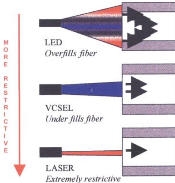
Figure 1. Depiction of the differences between overfilled and restrictive launch in multimode fibers
